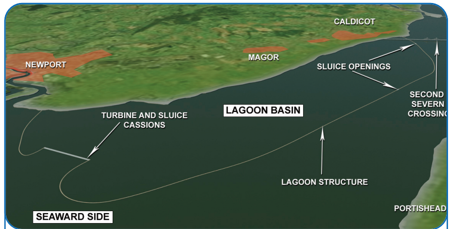
A shore-linked tidal lagoon as it might appear on the Welsh bank of the River Severn.
